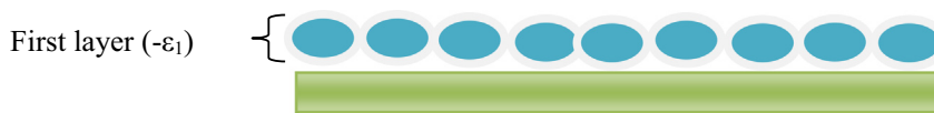
Fig. 1. Schematic illustration of the distribution of the molecules adsorbed on a solid according to the monolayer model with single energy.
